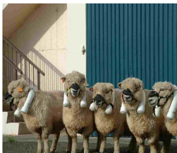
Sheep harnessed to measure methane production using the SF6 tracer technique
